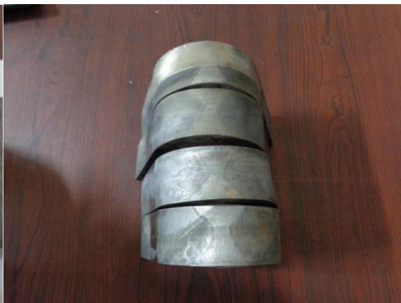
5B- Side bend tested after macro etching
