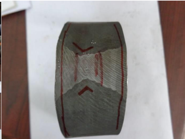
4B- Hardness tested sample after macro etch
