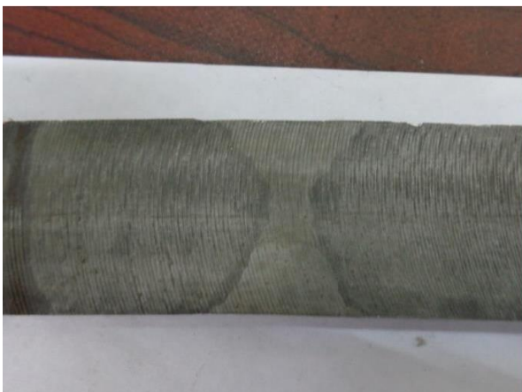
5A – Macro-etched weld sample
