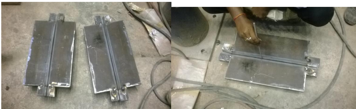
Test coupons fitment, root-gap inspection
