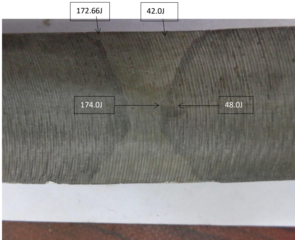
Charpy V notch location and Average impact strength
