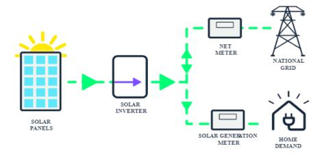
Figure 16. On-grid Solar PV system Source: Deege Solar, UK
