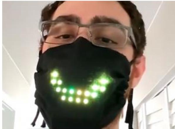
*Figure 74 LED face masks activated by voice Source (Demaral 2020)*
