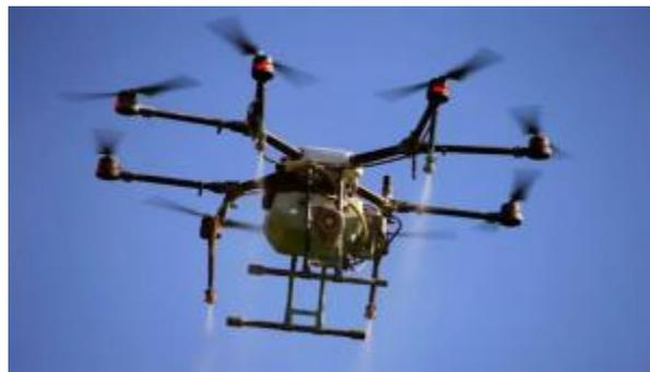
*Figure 77 Robotic aircraft that spray disinfectant Source (Demaral 2020)*
