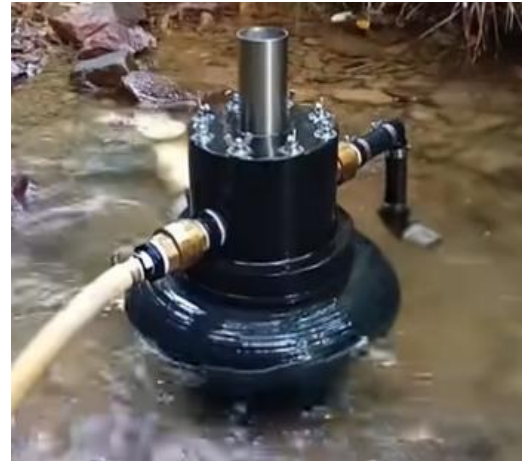
Figure 3.21: Sectional view of Bunyip Pump (left) and its photographic view (right). (Source: left, redrawn from [32], right [33])
