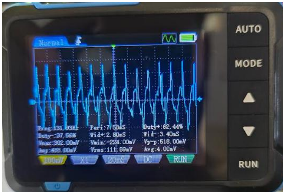
Figure 11 - Oscilloscope captures: raw diode noise and post-amp output
